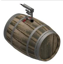
The BRA Flex PR.000.031 hand-held device for cleaning barrels at the storage location with electric drive consists of a cleaning head, an electric motor and a connecting pipe with a flexible squeegee.
